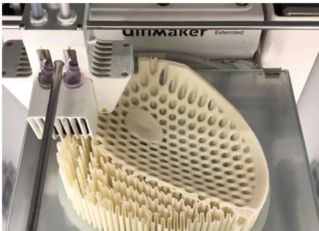
Fig. 6 The biomodel is created by selectively depositing melted PLA layer-by-layer in a predetermined path
